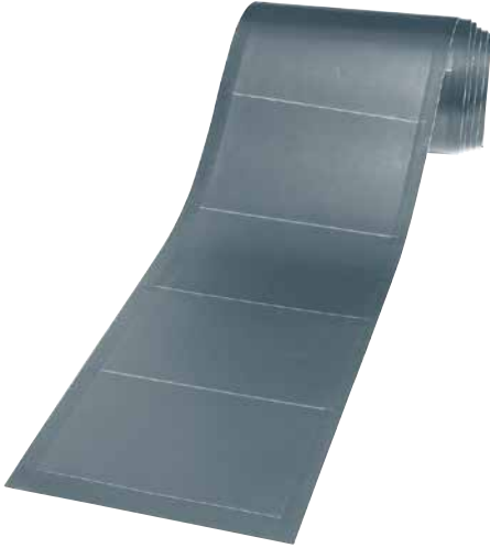
Figure 1.10. This product, known as PV laminate, is a plastic-coated flexible material that adheres to standing seam metal roofs. It’s best applied to new roof panels before they are installed on the building. PV laminate is not as sensitive to high temperatures as conventional silicon-crystal modules used in most solar systems. Credit: Uni-Solar.
