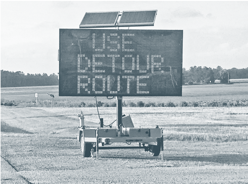
Figure 1.5. This electronic road sign is powered by a small solar array.
