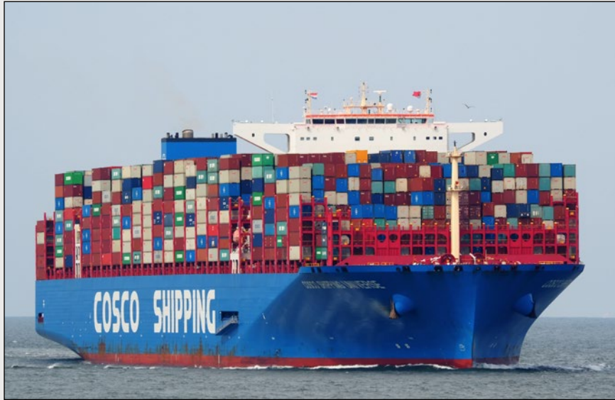
FIGURE 5.32. COSCO Container Ship "Universe Class," 400 meters long, capacity 21,337 20-foot containers, operated by a crew of 26. 70
