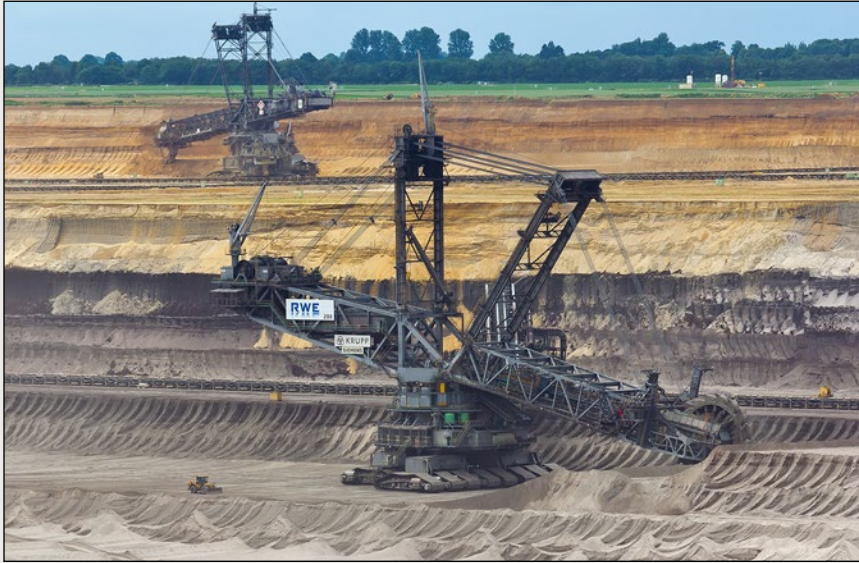
FIGURE 5.31. Bagger 288 (foreground) German open pit mining machine. Taller than the Statue of Liberty, heavier than the Eiffel Tower. A crew of three to four can mine 265,000 tons of fuel per day. 69 Note the bulldozer to the left for comparison.
