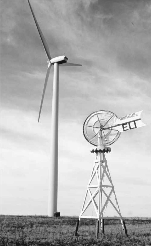
FIGURE 1.1. Water-pumping windmills like this one, photographed by Dan on a commercial wind farm in southeastern Colorado, were once common through the West and Midwest. The technology is so good that it hasn't changed in 100 years. Credit: Dan Chiras.
