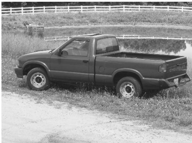
Fig. 1.1: My latest, most sustainable transportation: a former gas-engine truck that my brother-in-law and I converted to electricity. This vehicle is used for short trips to town and around the farm and The Evergreen Institute.
